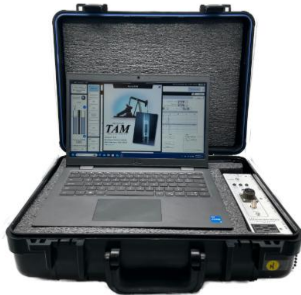
Figure 3. - Echometer Well Analyzer (Echometer Resigned, n.d.)
