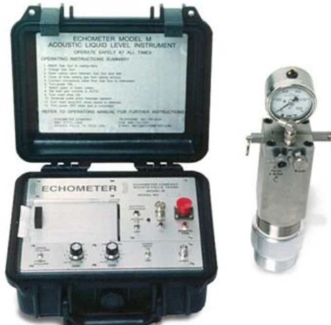
Figure 2 Powder-actuated Sonolog Model M (Echometer Model M Strip Chart Recorder - UPC Global, n.d.)
