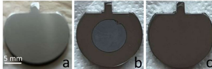
Figure 4 Sample surfaces a) before electrochemical tests, b) after electrochemical testing in pH 2.9 solution, c) after electrochemical testing in pH 6.5 solution
