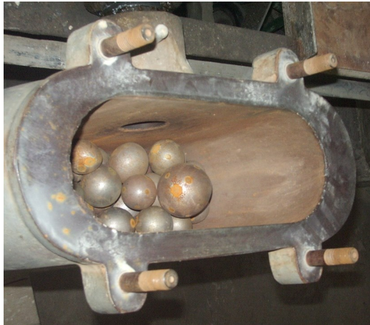
Figure 4 Denver laboratory mill (Deušić & Lazić, 2013)
