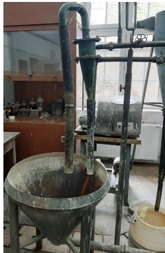
Figure 6 Laboratory setup for hydrocyclone testing
