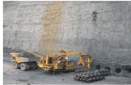
Figure 3 – Coal mining by rotary drilling and it load directly into truck
