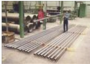
Figure 5 - Composite drill pipes laid on platform
