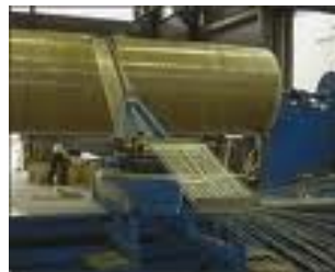
Figure 3 - GRE pipe – procedure of winding of glass fibers
