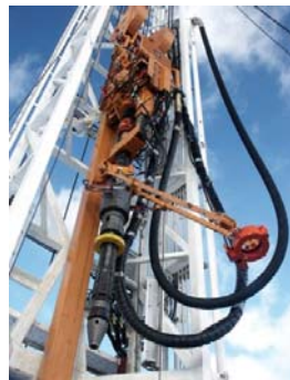
Figure 9 CDS connected to the top drive (Fontenot et al. 2005)
