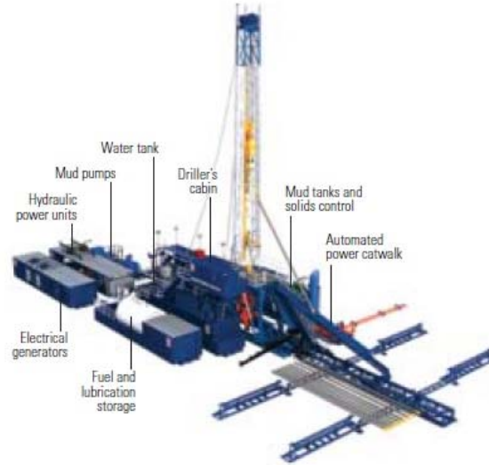
Figure 8 Automated Casing Drilling Rig (Fontenot et al. 2005)
