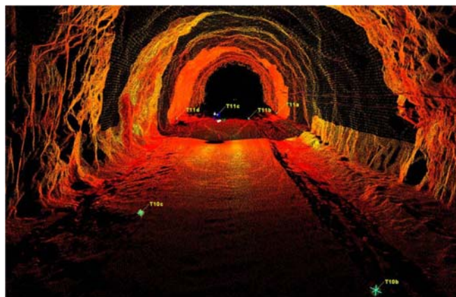
Figure 9 - Point cloud of the scanned tunnel ( http://www.gess.co.za )
