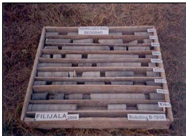
Figure 2 - Borehole B-19/06 with excavated Pannonian marl within the depth interval 96 – 104 m
