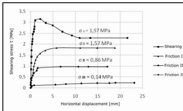
Figure 7 - Results of shearing experiment - charts of shearing and friction
