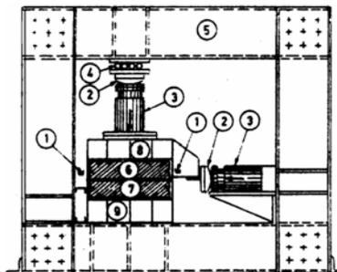
**Figure 6** - Device for carrying out shearing along fractures on cylindrical samples:
