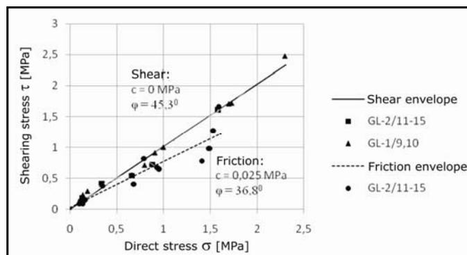
Figure 8 - Charts of shear strength and friction for "contour line" type of discontinuity that do not contain clay in the infilling
