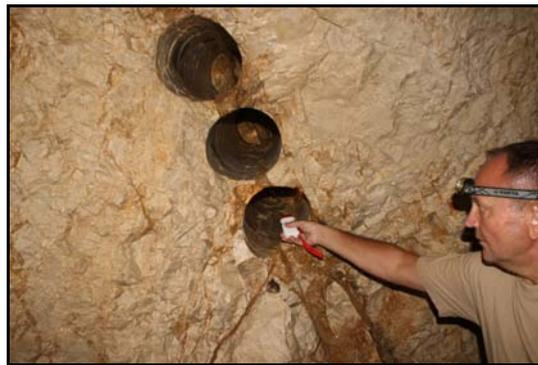
**Figure 5** - Locations where cylindrical samples of the rock mass along the fracture were taken in order to carry out one series of testing
