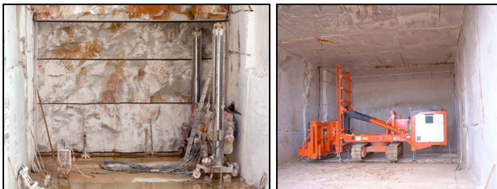
Figure 4 - An old and a new model of the chain saw machine for underground mining. Left: the Fantini G.70 model on fixing pillars (Primavori, 2005). Right: the new Fantini GU70/R model (Kortnik, 2009a)
