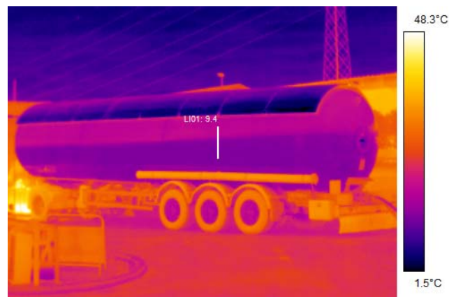
Figure 6 - Thermogram of the tank filled with gas ( www.flir.com )
