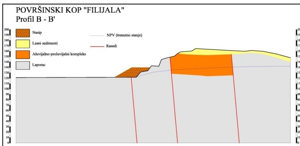
Figure 15 - Appearance of section B - B' with applied slope stabilization measures
