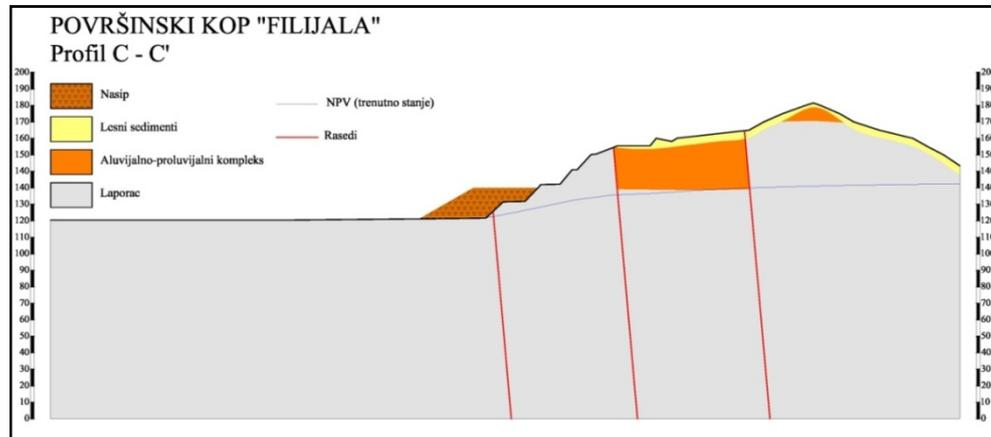
**Figure 16** - Appearance of section C - C' with applied slope stabilization measures
