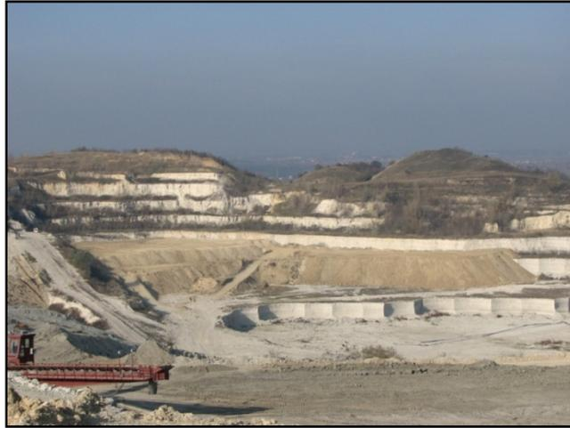
**Figure 20** - Appearance of counterweigh embankment in northwestern slope area at open pit "Filijala"
