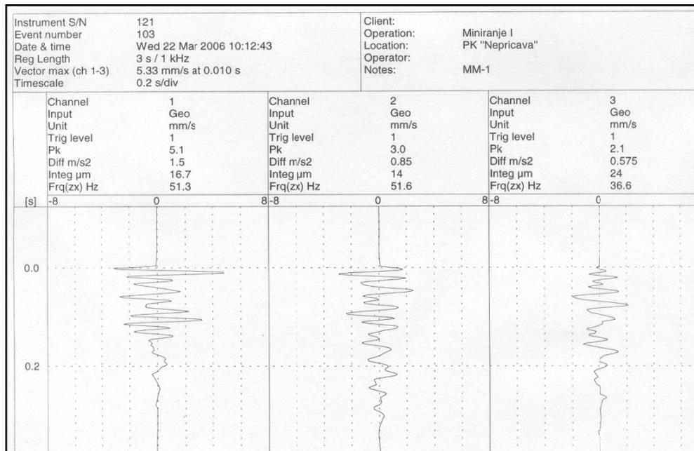
Figure 1 - Velocity shot for blasting No.I, measurement point MM-1
