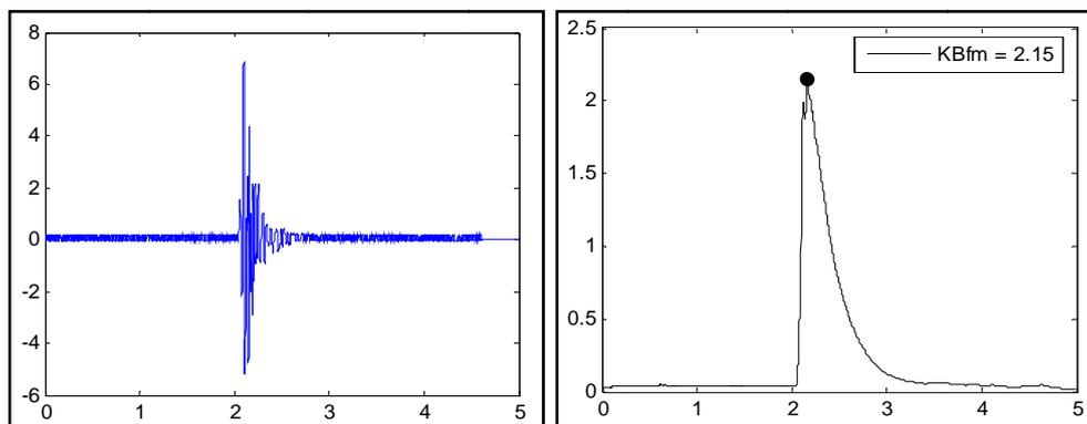
Figure 2 - Value of  $v_v$  and  $KB_{fm}$  components. Blasting No.I, measurement point MM-2
