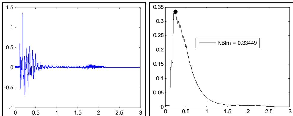
**Figure 4** - Value of  $v_v$  and  $KB_{fm}$  components. Blasting No. III, measurement point MM-1
