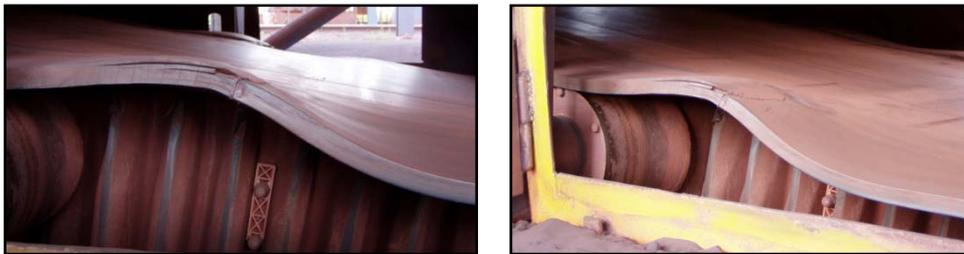
**Figure 2** - Strong wear of the FLEXOWELL belt
