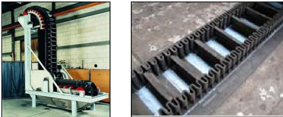
**Figure 1** - The FLEXOWELL belt conveyor ([www.meteoro.pt](http://www.meteoro.pt); [www.vvvmost.com](http://www.vvvmost.com))
