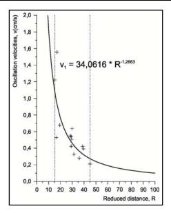
Figure 2 - Graphic survey of soil oscillation law curve in "Nepričava" Open Pit Mine
