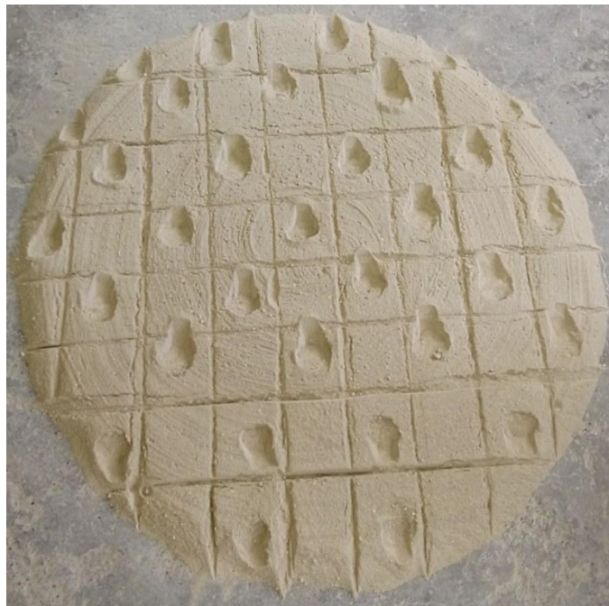
Figure 2 Cake after sampling using the checkerboard method
