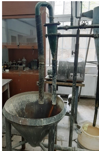
Figure 6 Laboratory setup for hydrocyclone testing
